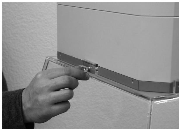
**2)** Unscrew the wing screws and remove the CleanZone system from the hood.
