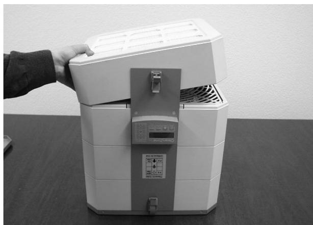
**4)** Remove the grill and lift out the top filter holder containing the pre-filter.
