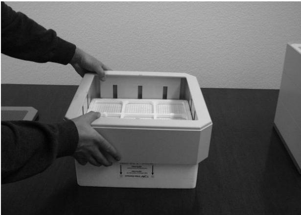
7) Lift the filter holder off the filter. Carefully dispose of the used filter in accordance with local regulations.
