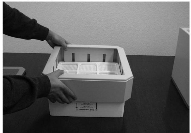
**6)** Lift the filter holder off the filter. Carefully dispose of the used filter in accordance with your local regulations.
