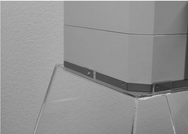
**1)** Lift the CleanZone system on top of the acrylic hood and place it carefully within the placement tabs at the top edge of the hood.
