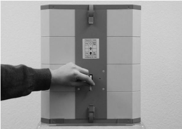
**1)** Take the flat-band cable on the front of the system and slide it through the gap of the control panel housing.
