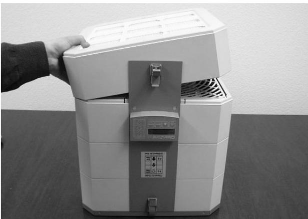
9) Replace the filter clips and push each down tightly. Turn the filter holder around and place it on top of the system.
