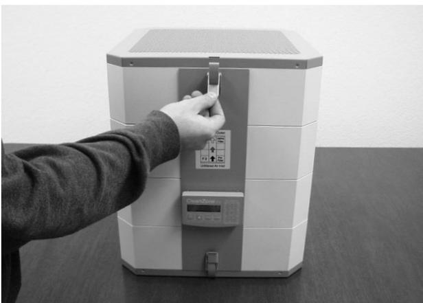
11) Close both latches. Don't forget to reset the filter life LED (see Chapter 2.7 )
