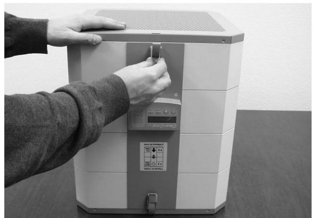
10) Replace the grill and close both latches. **IMPORTANT: Ensure that you replace the system onto the hood the correct way around for your application purposes. Don't forget to reset the filter life LED (see Chapter 2.7).**
