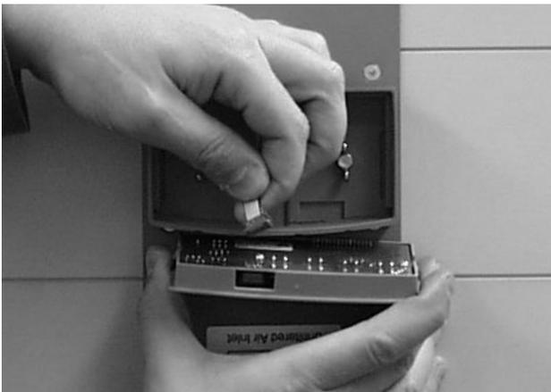
**3)** Plug the red clip attached to the flat-band cable into the red socket on the side of the touchpad.
