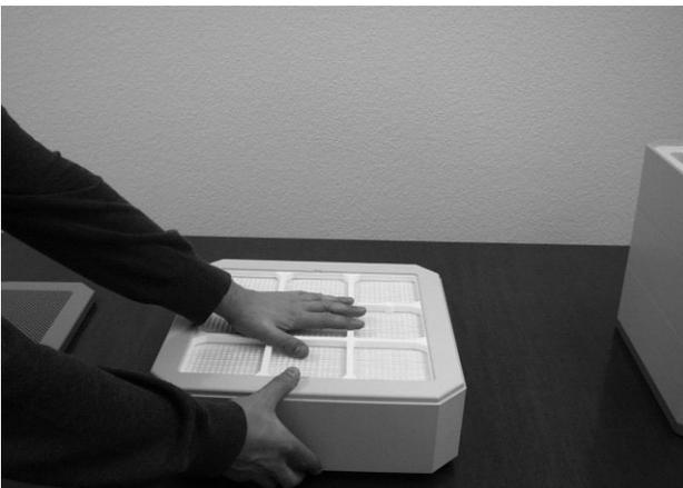
**5)** Turn the filter holder around and carefully press down on the filter element with the palm of your hand.
