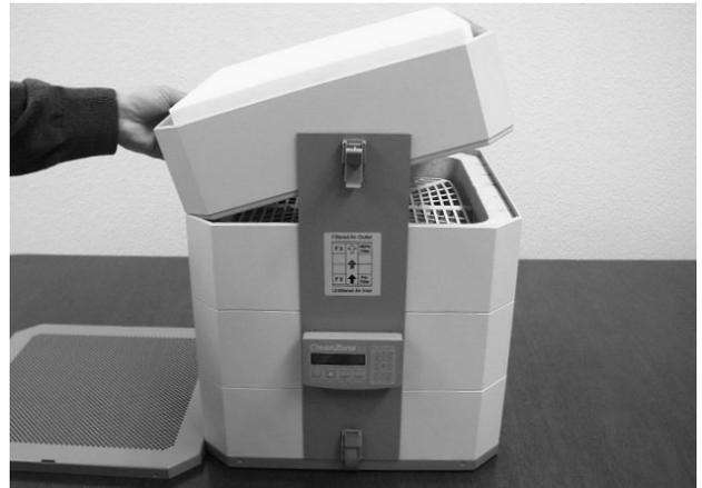
**4)** Remove the grill and lift out the top filter holder containing the HEPA-filter.
