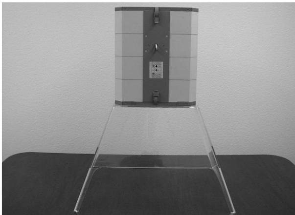
**3)** The CleanZone is now securely fixed to the hood. Note: To relocate the CleanZone, it is advisable to remove the system from the hood.
