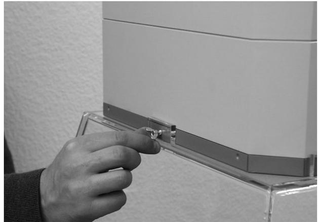
**2)** Screw the supplied wing screws through the pre-drilled holes on both sides of the hood into the metal frame.
