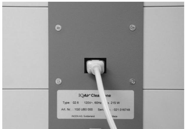
**6)** You can now connect the CleanZone to mains power with the supplied power cable.
