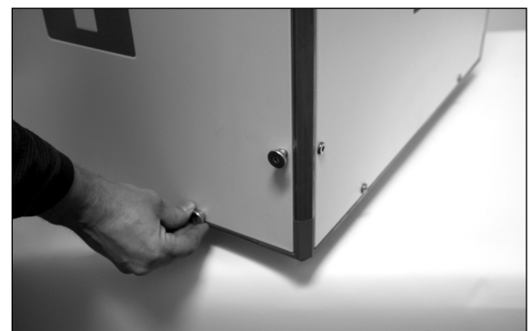
7. Install the filter access panel by using the eight large thumbscrews.
