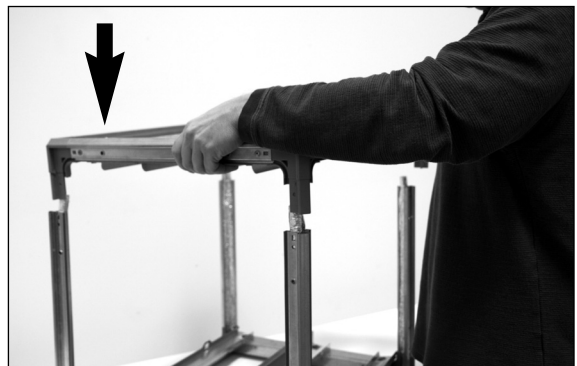
8. After you have the system in its new location, reinstall the top frame to the bottom frame.
