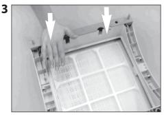
Press down until the mounting rail snaps into place. Repeat with second rail.
