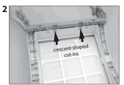
Place the mounting rail on the purifier's base so that the holes line up with the black connector pins on the base. The cut-ins should face the center of the unit.
