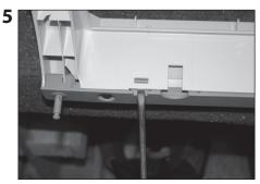
Using a flat-head screwdriver, press firmly into the slotted tab.
